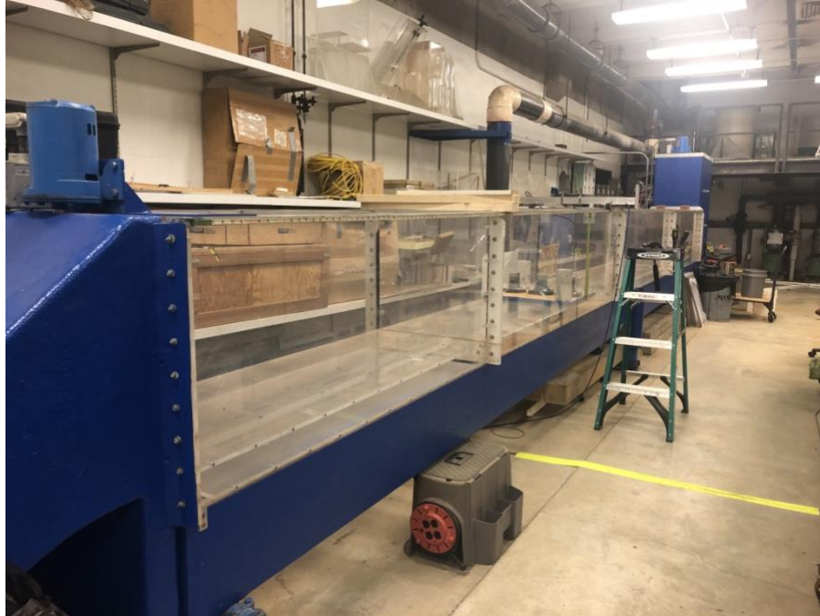
Figure 3.5 Flume channel used for erosion test
